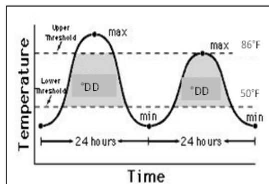
**Figure 2.** Accumulation of degree-days within upper and lower development thresholds of SWD using the single sine method. Modified from:
