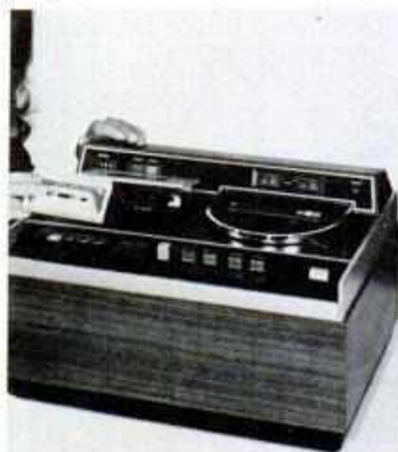
MATSUSHITA has developed a color picture cassette player that stores up to 1,000 color still pictures on a normal C-60 audio cassette.
